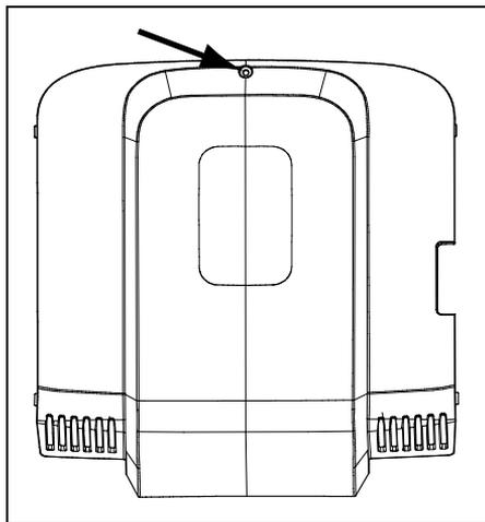
**Figure 19: Screw location for back cover of PVS**
