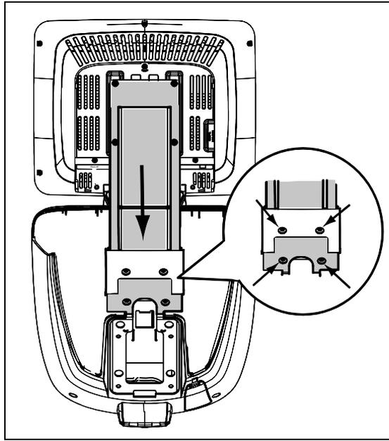
**Figure 22: Attaching the PVS bracket to the console**
