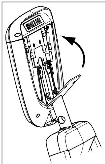
**Figure 4: Tilting console forward on console mount hook**
