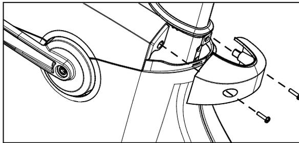
**Figure 10: Rear cover removal**
