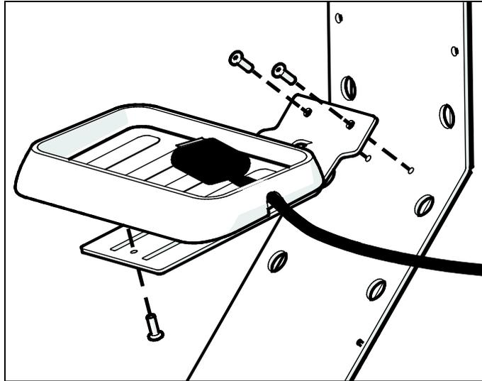
**Figure 20: Installing the iPod / iPhone tray and bracket**
