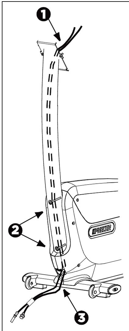
Figure 13: Threading the cables for the upright bike
