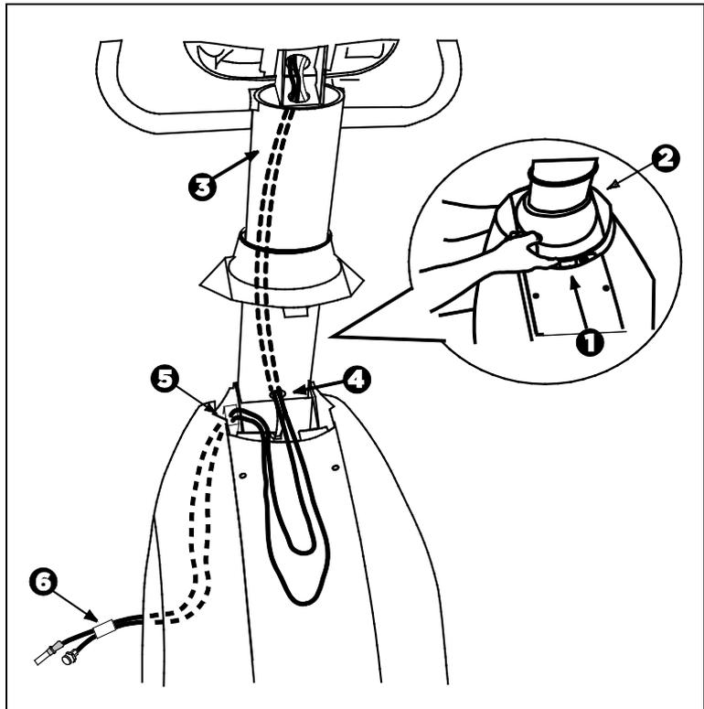
**Figure 14: Rewiring the climber**
