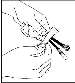
**Figure 5: Taping cables together**
