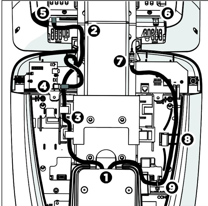
Figure 33: Routing the power and television cables
