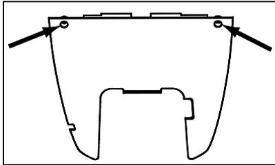
**Figure 16: Screw locations for back cover of console**
