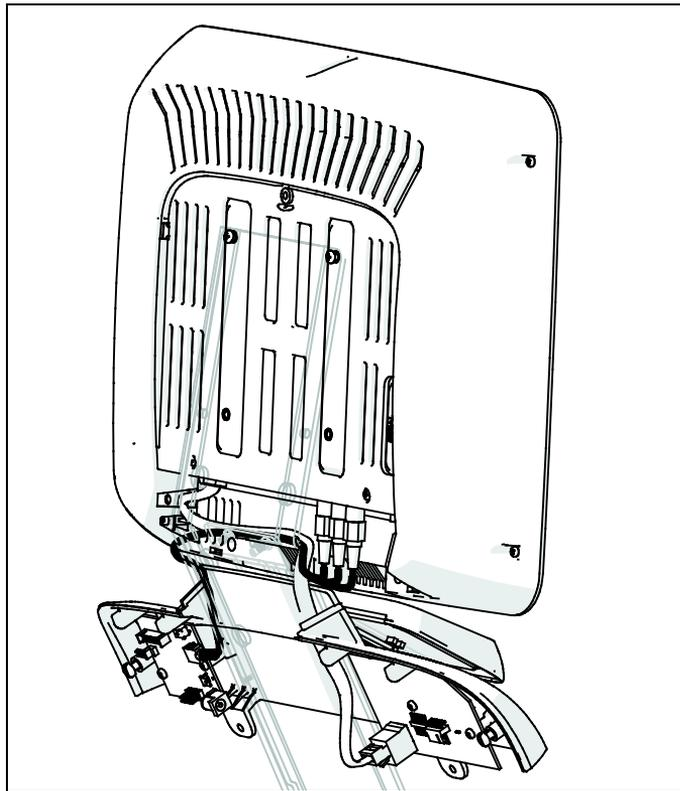
**Figure 31: Threading the communication and RCA audio/video cables**
