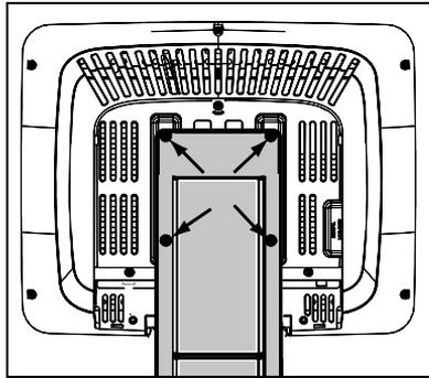
**Figure 21: Attaching the mounting bracket to the PVS**
