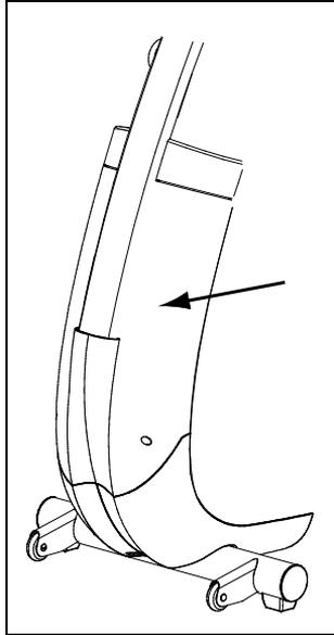
**Figure 15: Remove the front panel**
