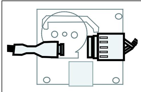
**Figure 30: Connecting the audio plug and grounding cable**
