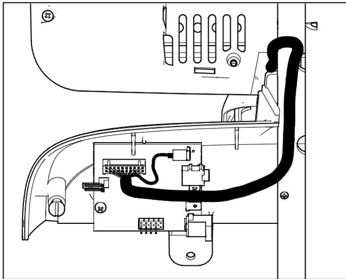
**Figure 32: Connecting the iPod/iPhone interface cable**
