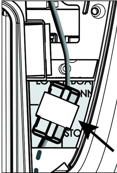
**Figure 27: Proper positioning of ferrite bead**
