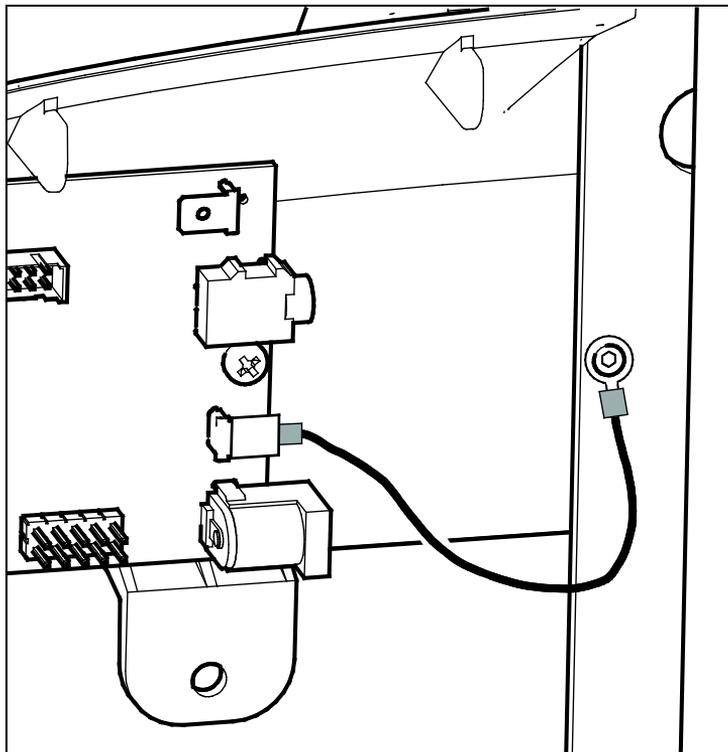
**Figure 24: Grounding the PEP interface board**
